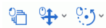
Figure 3.16: The tools activated with the left, the middle and the right mouse button respectively (from left to right)
