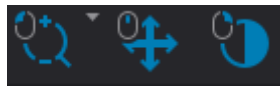
Figure 1.27: The tools activated with the left, the middle and the right mouse button respectively (from left to right)
